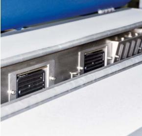
Modular hot air vulcanisation channel designed for energy-efficient and flexible vulcanisation of silicone.
