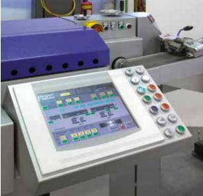
Hot air vulcanising channel with microwave (UHF) support designed for ultra fast profile cross-linking at high production speeds and for high demands on profile surface quality and sponge rubber profile cell structure, also rapid profile geometry stabilisation.
