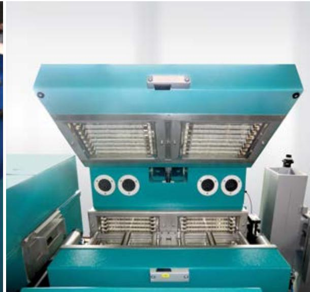
Through the use of special short-wave infrared emitters, excellent profile surfaces as well as early dimensional accuracy are achieved with both solid and sponge rubber products.
